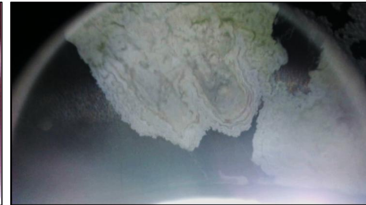
Urea deposit internal endoscope pictures sample
