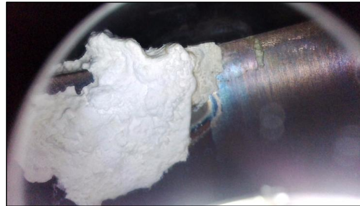
Urea deposit internal endoscope pictures sample
